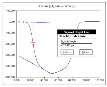
FIGURE 3.7: MEASURING THE HEIGHT OF A SIGMOIDAL FEATURE
