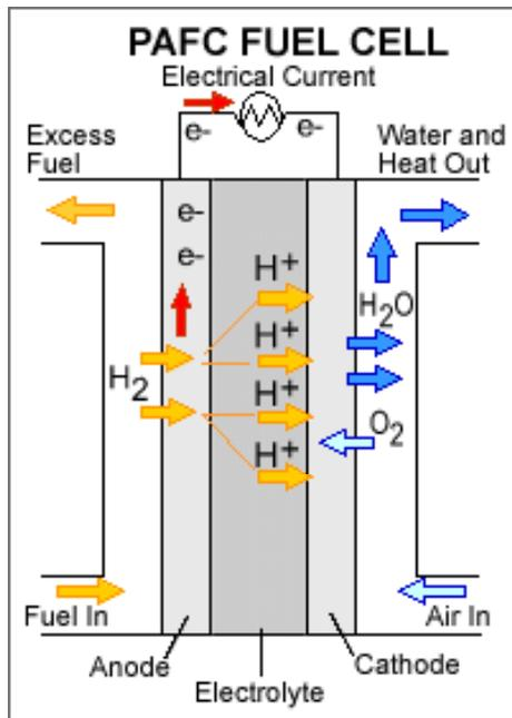
Phosphoric acid fuel cells use liquid phosphoric acid (H<sub>3</sub>PO<sub>4</sub>) as an electrolyte—the acid is contained in a Teflon-bonded silicon carbide matrix—and porous carbon electrodes containing a platinum catalyst.
