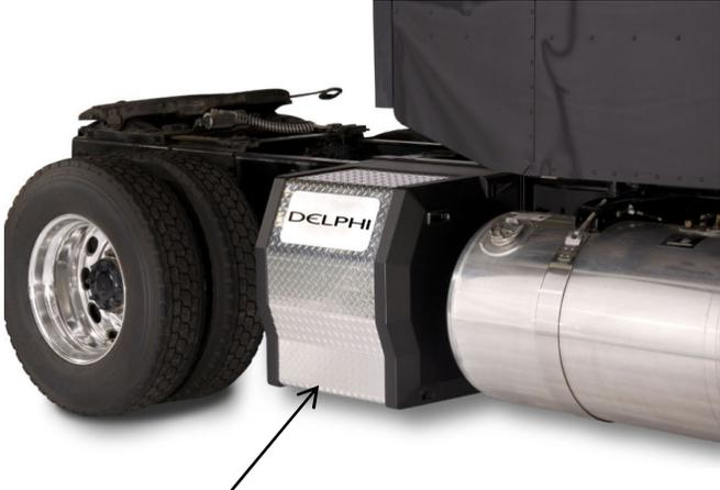
Delphi offers its solid oxide fuel cell (SOFC) technology as an **auxiliary power unit (APU)** to provide up to 5 kW (6.7 hp) of electrical power for use on commercial vehicles during extended idling periods. <http://www.sae.org/mags/sve/TOOLS/product/8402>
