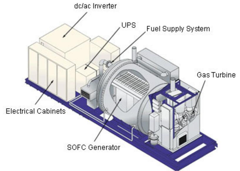
Since the SOFC stack operates at 1000°C it produces a high temperature exhaust gas. If operated at an elevated pressure, the exhaust becomes a hot pressurized gas flow that can be used to drive a turbine.
