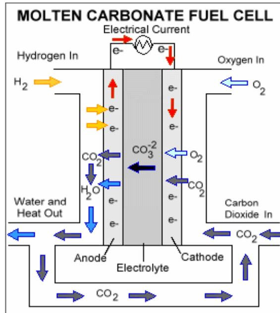
MCFCs are high-temperature fuel cells that use an electrolyte composed of a molten carbonate salt mixture suspended in a porous, chemically inert ceramic lithium aluminum oxide ( $LiAlO_2$ ) matrix. Because they operate at extremely high temperatures of  $650^\circ\text{C}$  (roughly  $1,200^\circ\text{F}$ ) and above, non-precious metals can be used as catalysts at the anode and cathode, reducing costs.
