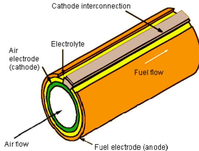
In a tubular SOFC design, air flows through the interior of the cell, and fuel flows on the outside of the cell. At elevated temperatures, the oxygen in the air ionizes and the resulting ions flow through the electrolyte and combine with the fuel on the cell's exterior. This is an electrochemical reaction, so electrons are released. With proper connections, they can flow through an external circuit as electricity.
