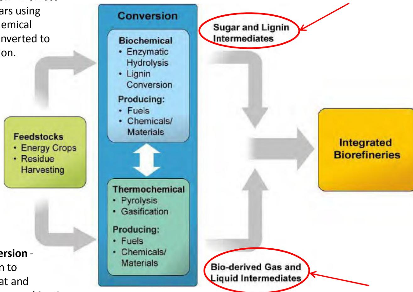
**Thermochemical Conversion** - Biomass is broken down to intermediates using heat and upgraded to fuels using a combination of heat and pressure in the presence of catalysts.
