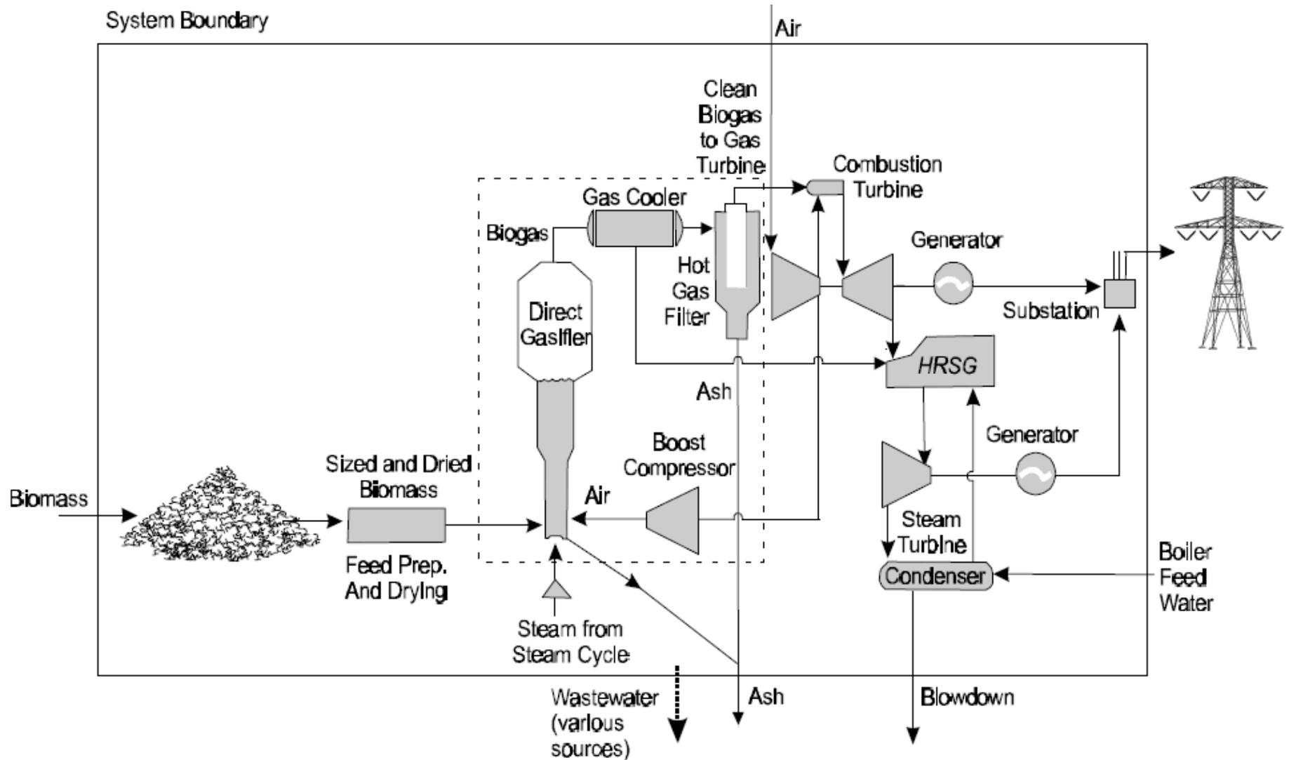
Biomass gasification combined cycle (BGCC) system schematic.
