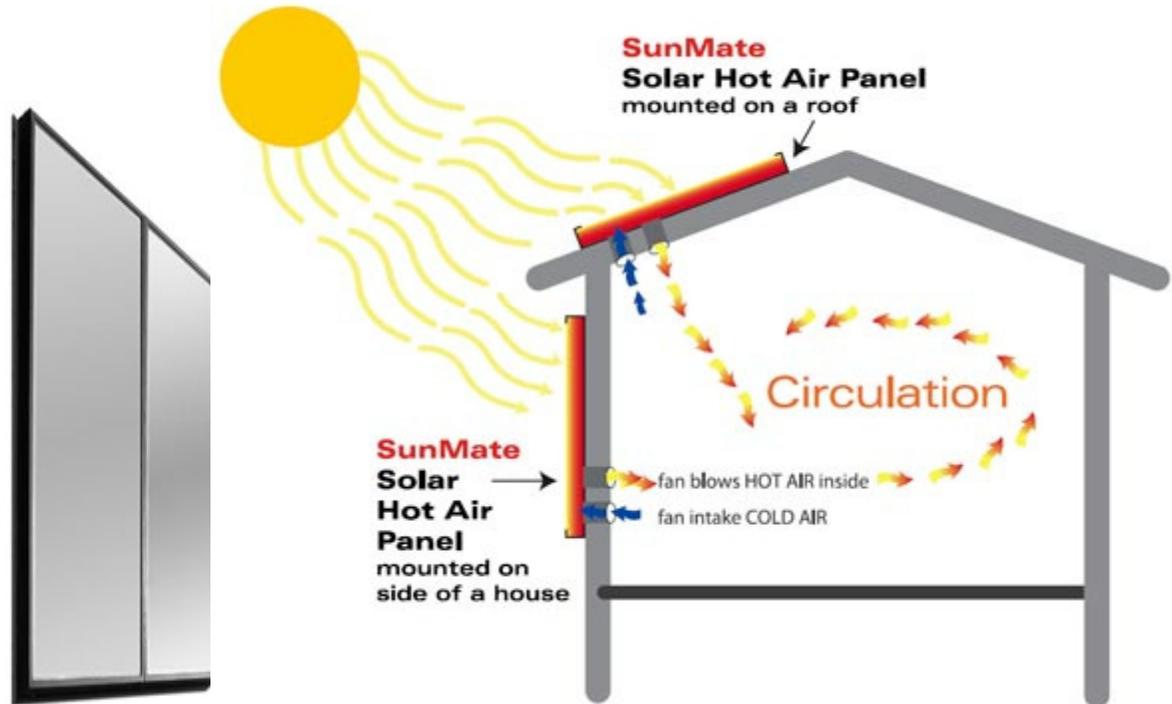
Pulls cool air from your home, channels it through the absorber plate where it's warmed by energy from the sun, then circulates it back into your home. A built-in thermostat, automatically turns on a blower when the absorber plate reaches 110° F and shuts off the blower at 90° F.
