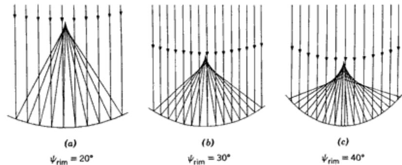
Focusing of parallel rays of light using circular mirrors with different rim angles
