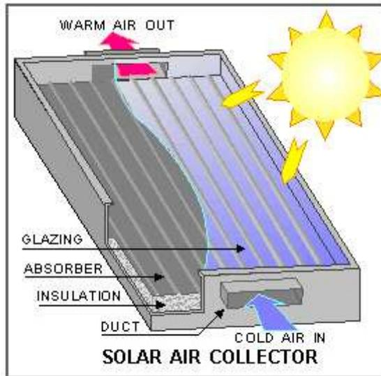
**Air based solar collectors use air instead of liquids as the energy transfer medium**
