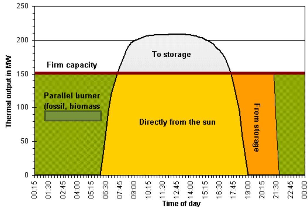
Typical output of a solar thermal power plant with two-hour thermal storage and backup heating system to guarantee capacity.
