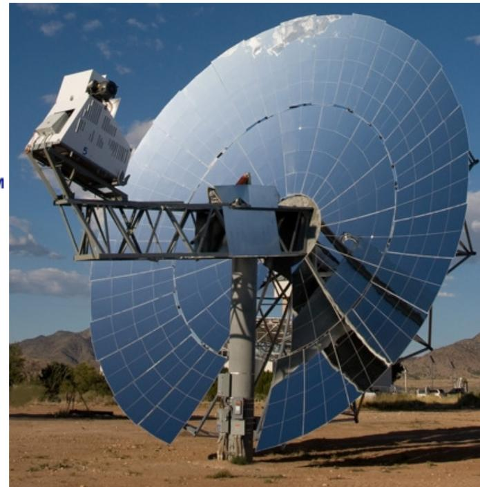
The SunCatcher™ is a 25-kilowatt-electrical (kWe) solar dish Stirling system which consists of a radial solar concentrator dish structure that supports an array of curved glass mirror facets, designed to automatically track the sun, collect and focus solar energy onto a Power Conversion Unit (PCU). The PCU is coupled with, and powered by, a **Stirling engine that generates electricity.**
