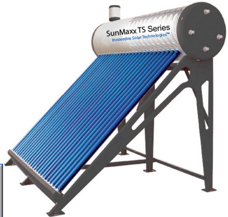
Water flows through the system when warm water rises as cooler water sinks. The collector must be installed below the storage tank so that warm water will rise into the tank. These systems are reliable, but contractors must pay careful attention to the roof design because of the heavy storage tank. They are usually more expensive than integral collector-storage passive systems.
