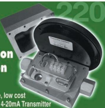
Model 220 now provides a simple, low cost Loop Powered 8-28 Vdc two wire 4-20mA Transmitter using the same CSA, UL & ATEX rated sensor and explosion-proof housing used on the Model 220 with switches. The transmitter with an industrial type terminal strip is housed in a heavy-duty, cast aluminum housing. Wiring access is through a 1/2" NPT port. Accuracy is  $\pm 2\%$  from 20% to 100% of full scale. Indicator accuracy is  $\pm 2\%$  and is independent of the transmitter.
