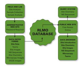
↑ Figure 2. RLMO Database Structure. This flow chart schematically illustrates the conceptual design of the database, following the process from field collection and analysis through data tables for administrative entry and public viewing.
