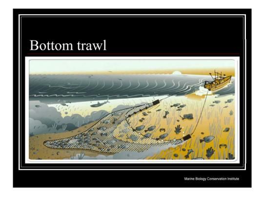
Many modern fishing vessels deploy larger, heavier gear than used in the past, allowing access to previously inaccessible fishing grounds. The bottom trawl shown here, for example, is held open by heavy doors (black rectangles in diagram) and dragged along the ocean floor. Some trawls are equipped with "rockhopper" gear (large rollers on bottom line in diagram) that allow bottom trawl nets to fish rocky, complex habitats where in the past gear would become damaged or lost.
